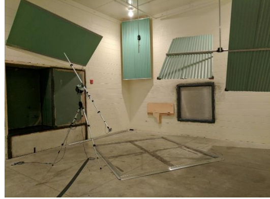
Fig. 2 – Reverberation room internal view.
