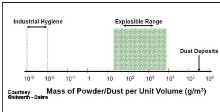
Fig. 4. Explosible range of a dust cloud.
