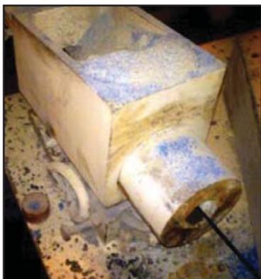
**Fig. 9. An example of lubricant becoming a dust issue from over filling the lubricant box.**
