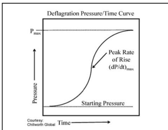
**Fig. 6. Deflagration Pressure Time Curve indicating the calculation of Kst.**
