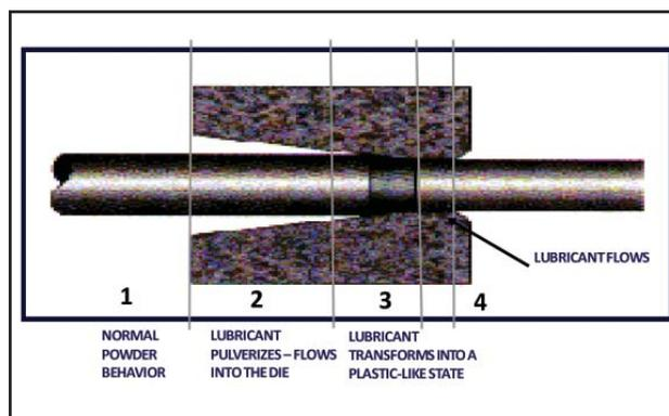
**Fig. 8. Large particles need to break into finer particles in Zone 2 to lubricate the die/wire interface in Zone 3.**
