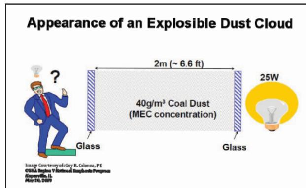
Fig. 5. A cloud of 40  $\text{g}/\text{m}^3$  of coal dust in air is so dense that a glowing 25 W light bulb can hardly be seen through a dust cloud of 2 m (6.6 ft) thickness.
