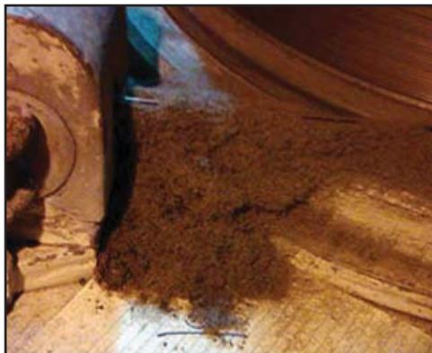
**Fig. 10. An example of incorrect lubricant choice resulting in significant feathering.**
